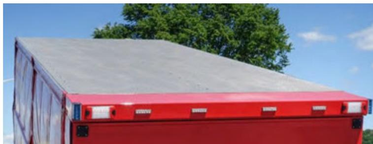
Abbildung 24: Festes Aluminiumdach in Alu-Gerstenkorn.
